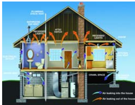
Arrows denote air leaking into or out of a house. Image: U.S. EPA
